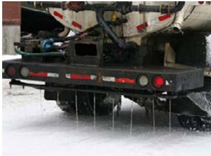
The use of de-icer instead of solids can reduce the amount of salt needed.
